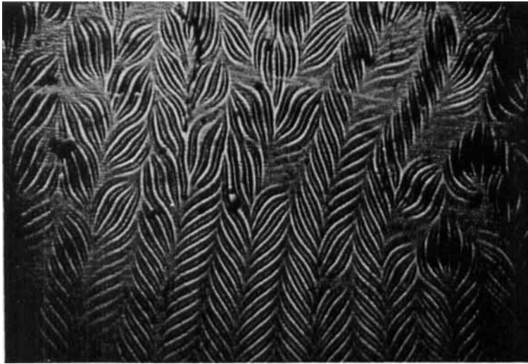
Figure 2. Typical aspect of the AC instability in the dielectric regime ("chevrons") in MBBA. V = 260 volt rms at 120 Hz. The distance between striations is 5 \mu\text{m} (thickness = 100 \mu\text{m} ). Picture taken a few volts above threshold; the striations are grouped in ribbons which shift slowly in alternating directions. This is one type of a further instability above threshold not considered in the model.
